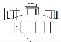
The EZ-FLO system uses push connect fittings to connect the clear and black 1/4" tubing to the cap.
