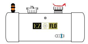
Step 7 -Turn on both shut off valves at the proportioning cap
