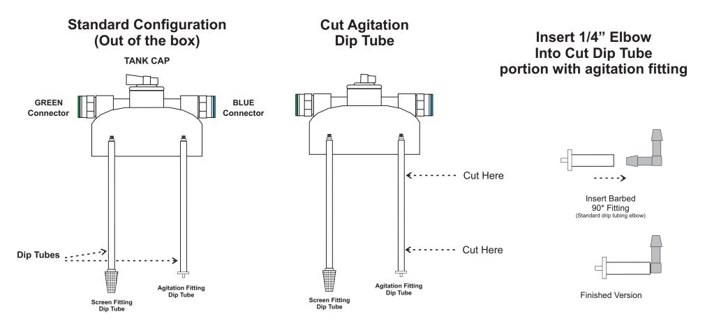
Cut the tube 1" from the top of the cap & cut 1" of tubing from the bottom of tubing leaving the agitation fitting in place
